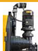
15 KW Main Motor
